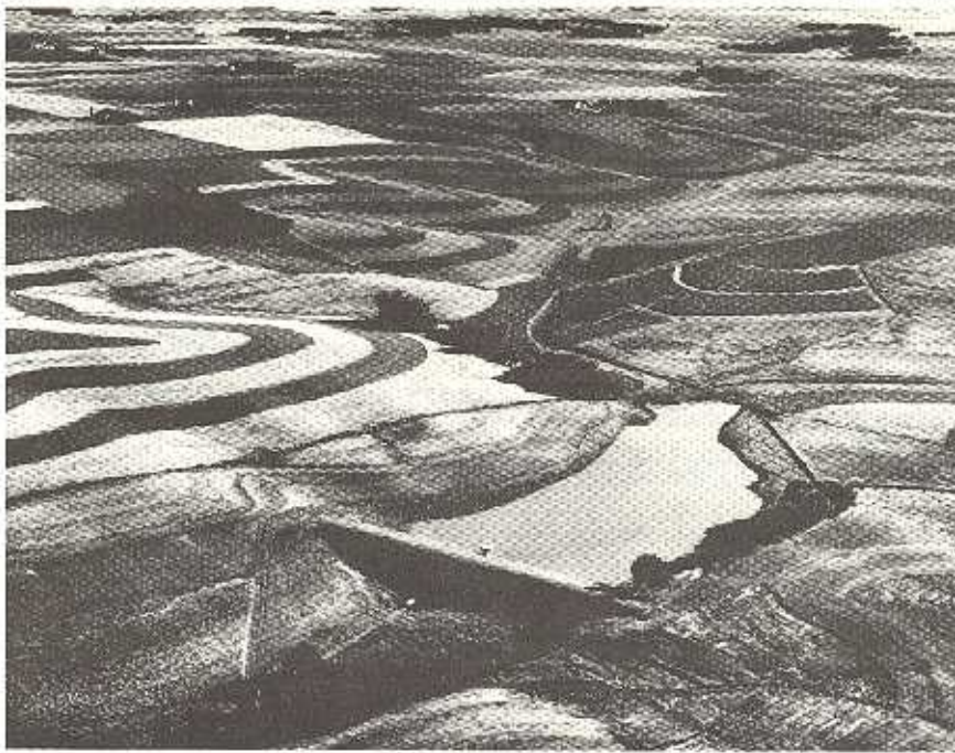
Diversions, terraces, waterways and contour stripcropping are major mechanical practices that keep soil and pollutants associated with it out of the water. (USDA - Soil Conservation Service)
