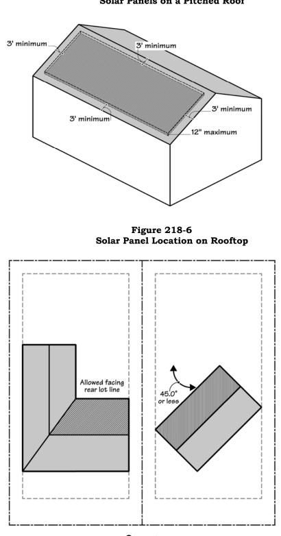
Figure 218-5 Solar Panels on a Pitched Roof
