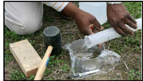
Figure 7: Preparing soil infiltration test
