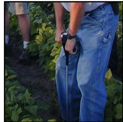
Figure 8: Applying slow, steady pressure when pushing penetrometer into soil
