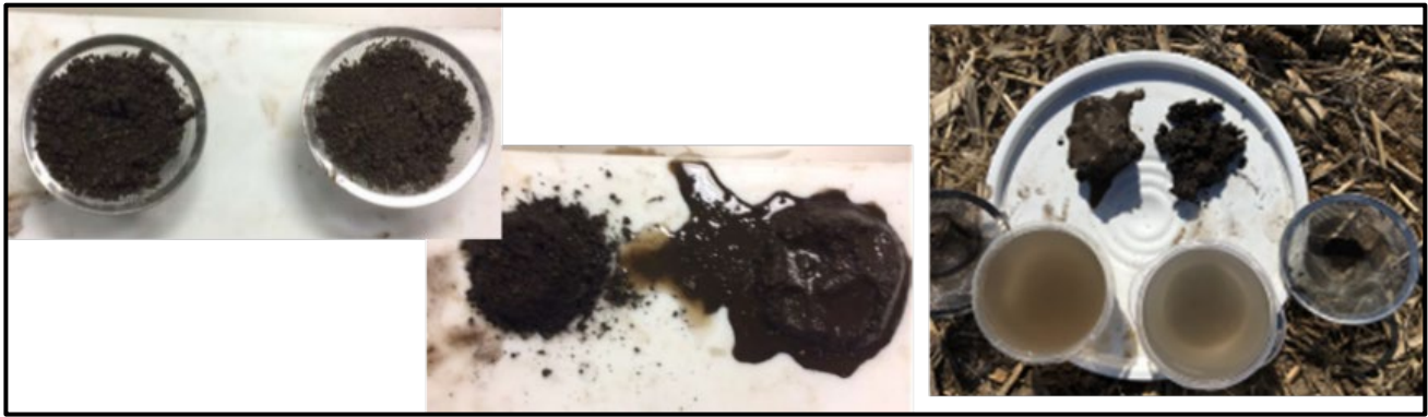
Figure 11: Sink strainer method showing water-stable aggregates on left and unstable aggregates on right
