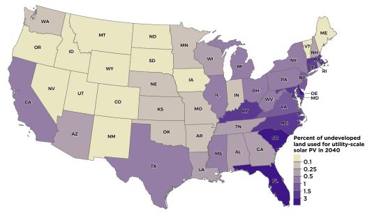
Figure 12. Projected percentage of undeveloped land remaining in 2016 that will be required for utilityscale solar photovoltaics (PV) energy generation facilities by state in 2040 in the Decarbonization with Electrification scenario of the Department of Energy's Solar Futures Study.134 Undeveloped land includes all land area except the urban and highly developed, lowdensity residential, and transportation categories of the Farms Under Threat geospatial dataset.
