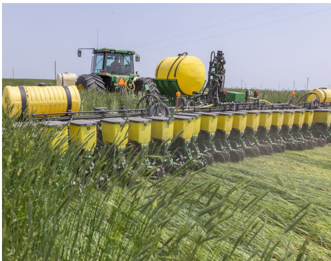
Using a roller crimper, either attached to the planter (as shown above) or a standalone unit, is one of the most effective strategies for season-long weed suppression.
