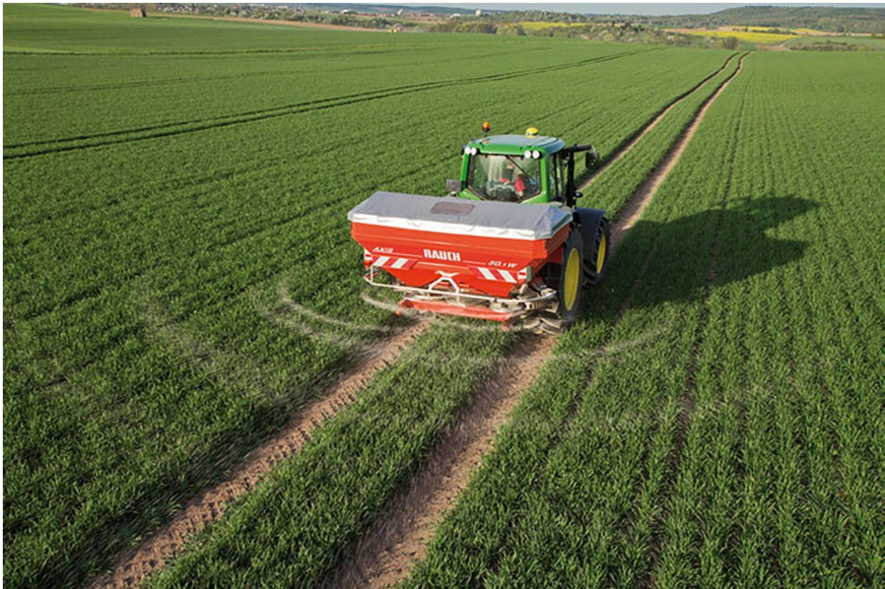
FIGURE 7. Example of farm machinery used to spread fertilizer on a field (Photo by RAUCH Landmaschinefabrik GmbH, CC BY-SA 3.0). 21
