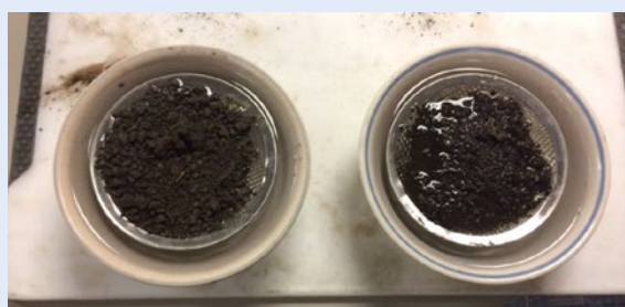
Step 3. Leave strainer of soil in bowl of water until each one is fully saturated. If necessary add extra water from the top to ensure both are fully saturated.
